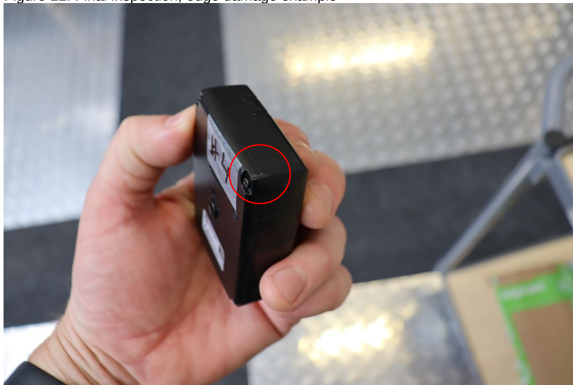
Figure 11: Final inspection, edge damage example
