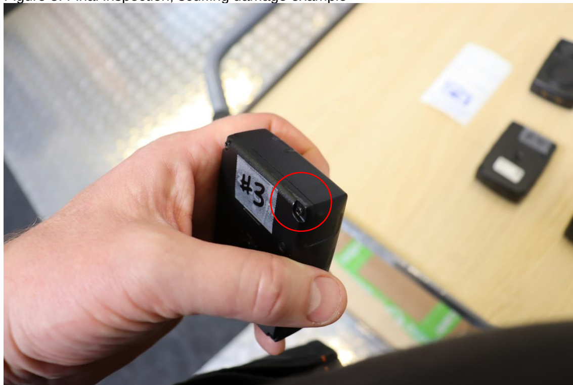
Figure 8: Final inspection, scuffing damage example
