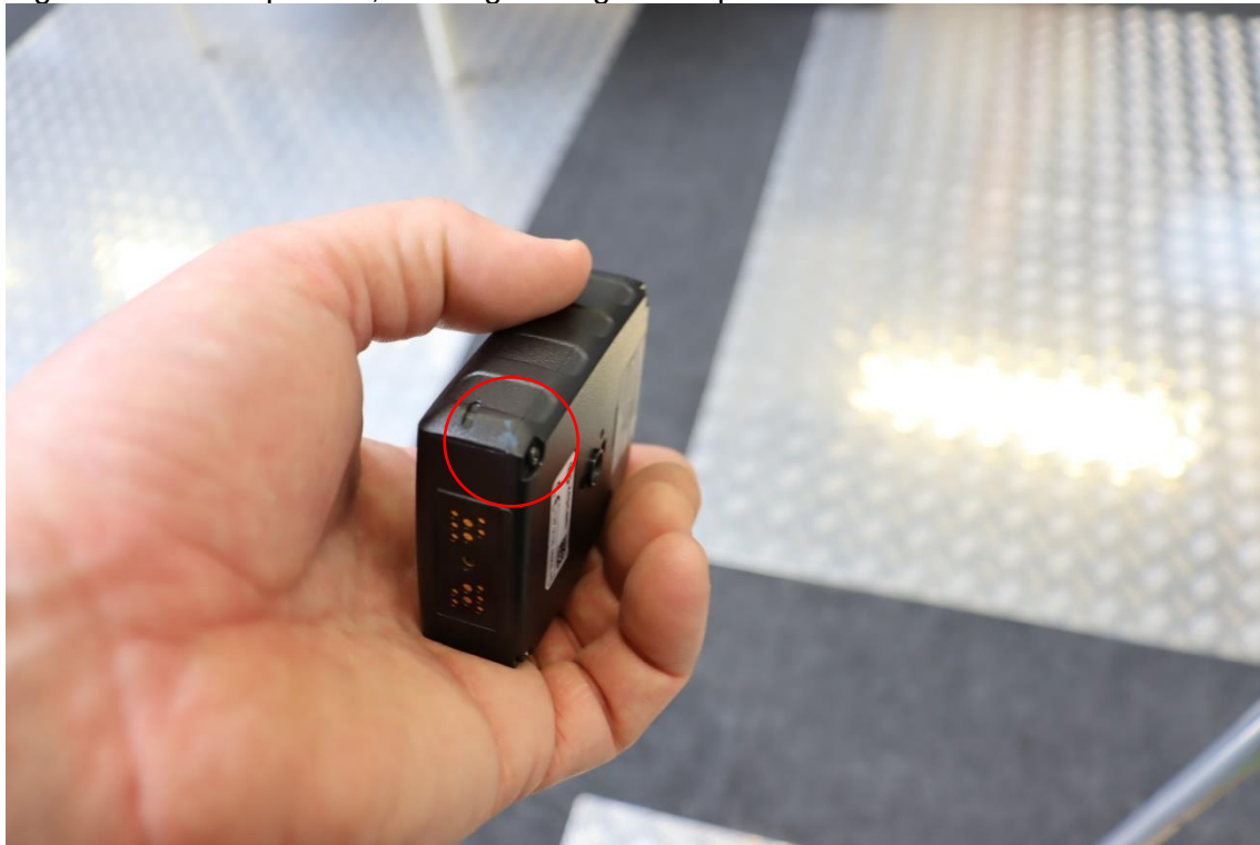
Figure 9: Final inspection, scuffing damage example
